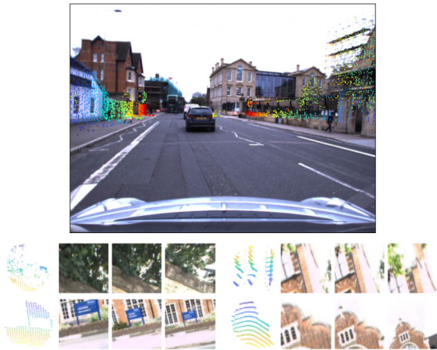
Figure 4: Project point cloud to image with ground truth pose. Four examples of our dataset. The first image of each example shows the ISS volume. The other three are some corresponding SIFT patches across multiple frames with different scale, viewpoint and lighting.
